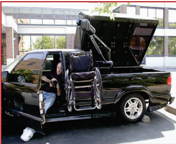
An example of a wheelchair lift for a pickup truck.
